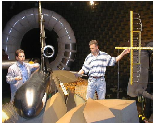
Aeroacoustic Wind Tunnel Cepra 19, 1:11 scaled 3D A320 wing
